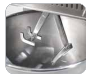
Braccia inox smontabili Removable stainless steel arms
